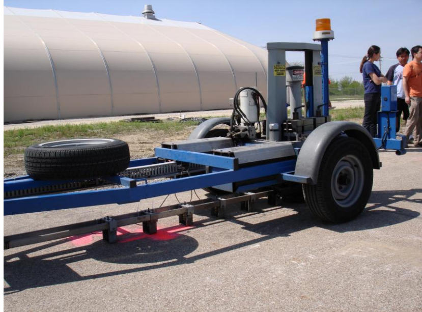
Figure 2.1. Dynatest Falling Weight Deflectometer device.
